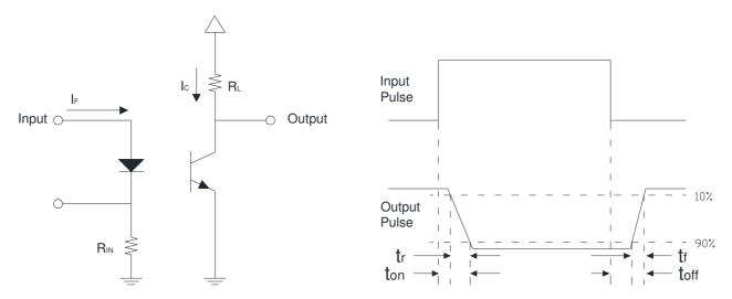
**Figure 13: Switching Time Test Circuits**
